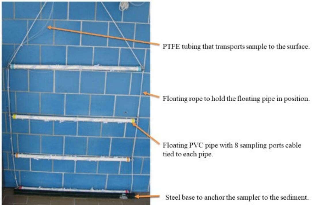
**Figure 2.** Sampler used to collect water from four heights in the water column inside and outside of the study plots.
