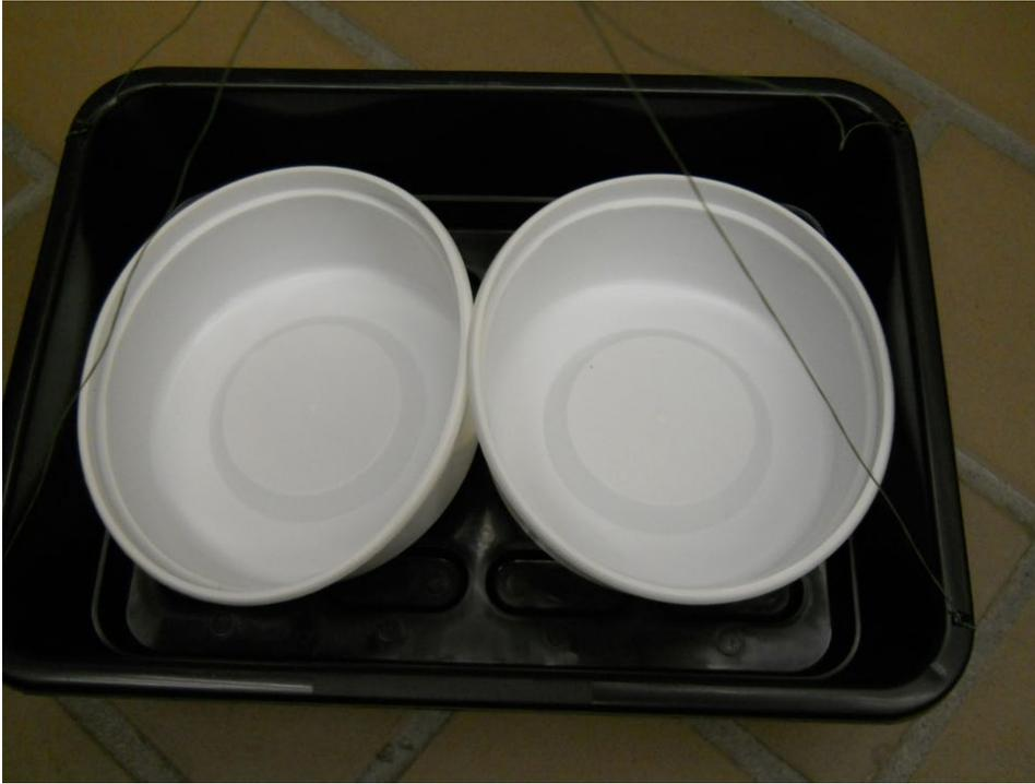
**Figure 4.** Sediment sampler: a tray (non-draining) with two non-draining 11-cm diameter x 4-cm deep dishes that were filled with sediment.
