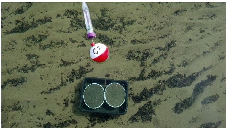
**Figure 3.** Deployed sediment sampler in the bay at the mouth of Hog Island Creek (Mackinac County, Michigan). Each samplers was marked by a small labeled float fastened to lines used to lower and raise the sampler.
