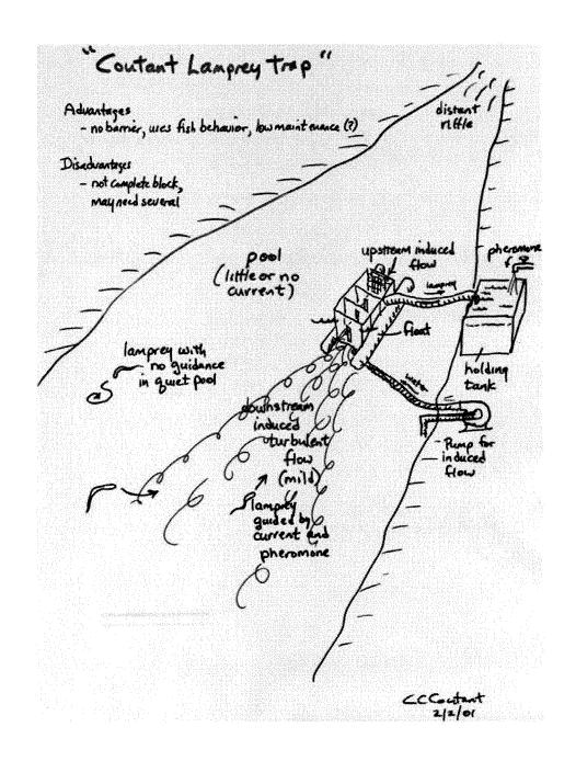
Figure 1. Schematic of the Coutant Lamprey trap
