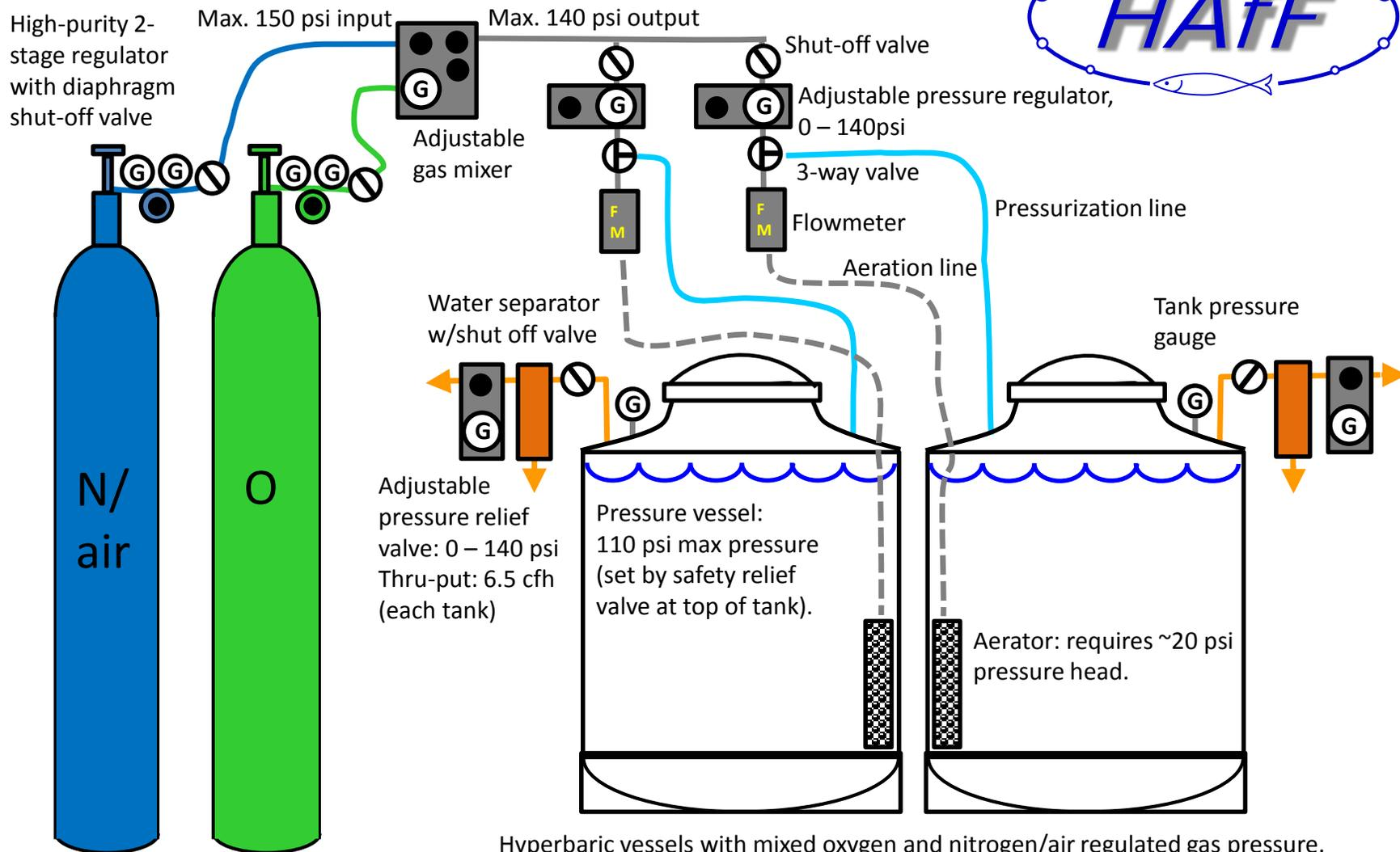
Hyperbaric vessels with mixed oxygen and nitrogen/air regulated gas pressure. Vessel pressure is regulated by adjustable precision pressure regulator in tandem with relief valve.
