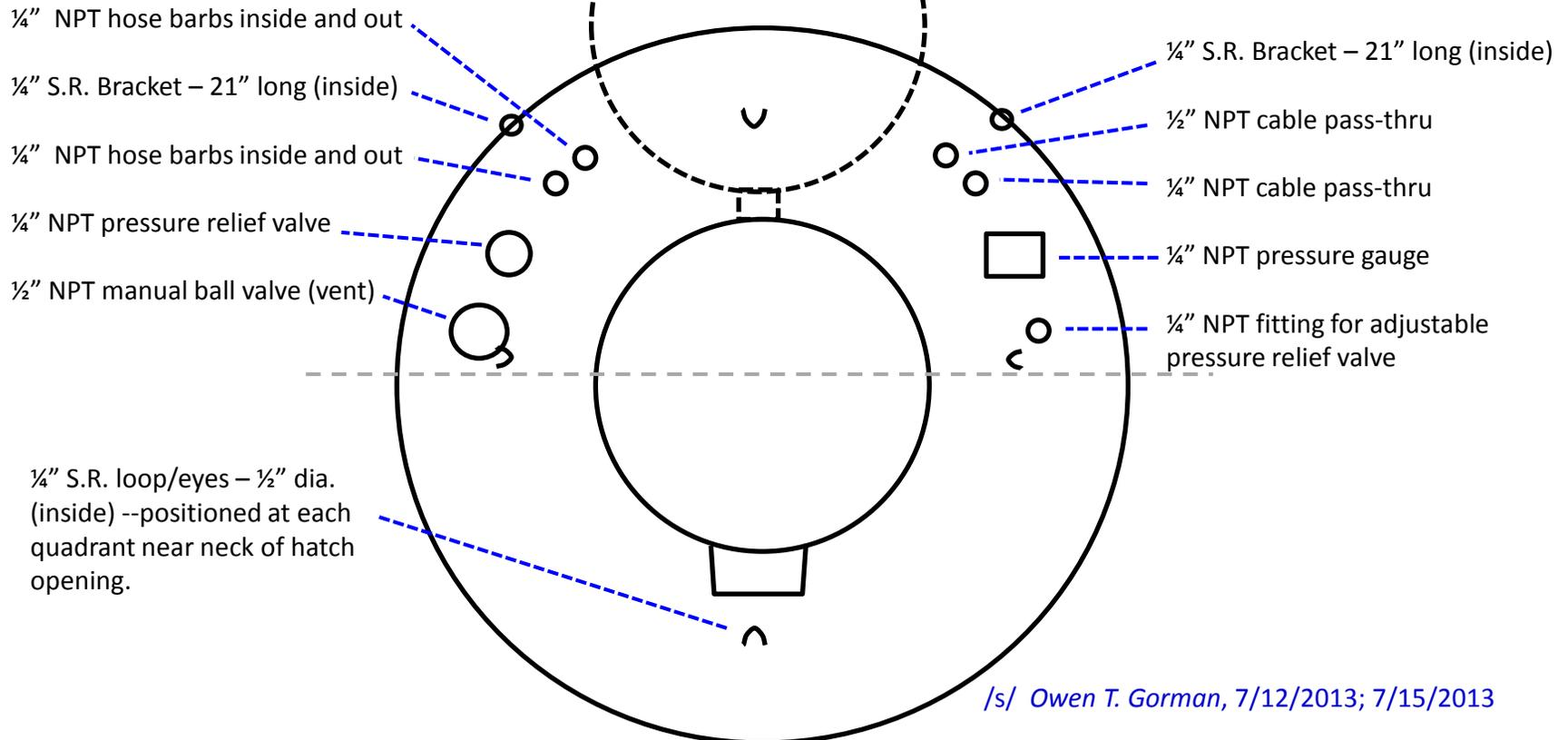
Vessel top: suggested lay-out of connections, pass-thrus, hatch hinge and lift handle
