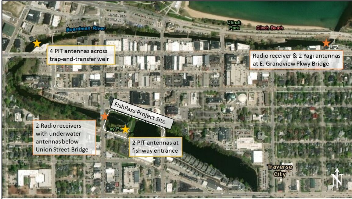
Figure 4-2. Locations of radio receivers with aerial directional Yagi and underwater omnidirectional dipole radio antennas, and PIT antennas in the existing Union St. Dam fishway and trap-and-transfer facility weir.
